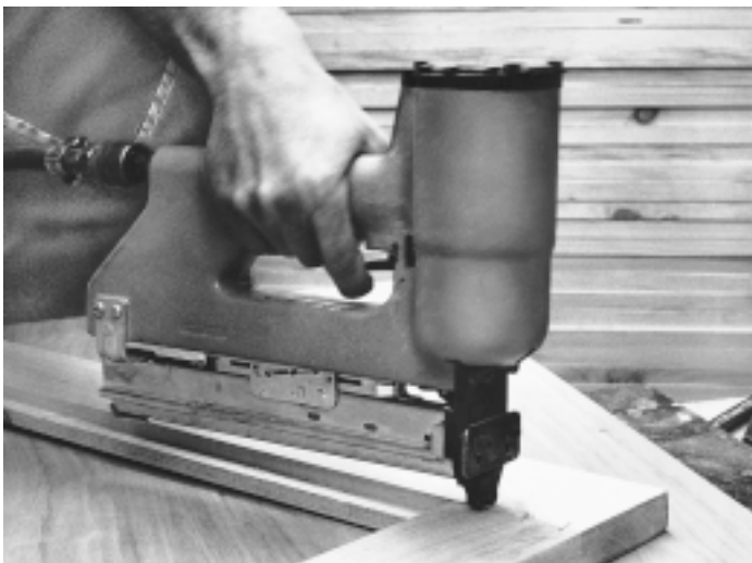
The SC1 & Senclamp performs a butt joint in a mirror frame application.
